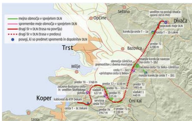
Figure 6: Track of the second railway line Koper - Divača
