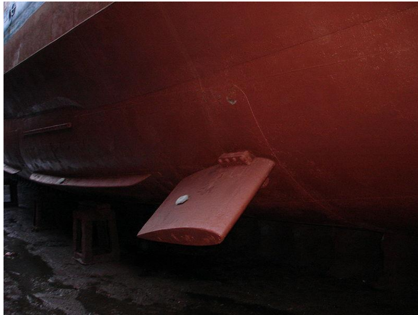
Figure 8: Photograph of passive fin stabilizers: a fixed fin stabilizer (front) and bilge keels.
