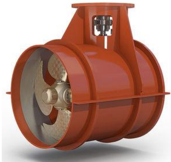
Figure 4: Tunnel thruster system
