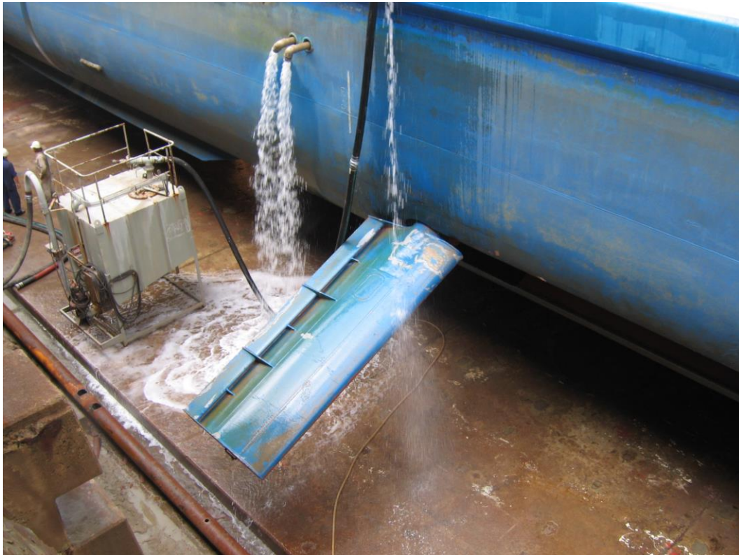
Figure 6: Photograph of Folding Fin Active Stabilizer of the cruise vessel in dry dock
