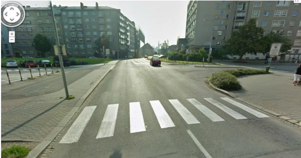
Figure 1: Single crossing, narrow street with turning vehicles, no traffic lights. Average speed: 28.2 km/h. Densities (cars/pedestrians: 3358/1903, ratio 1.76)
