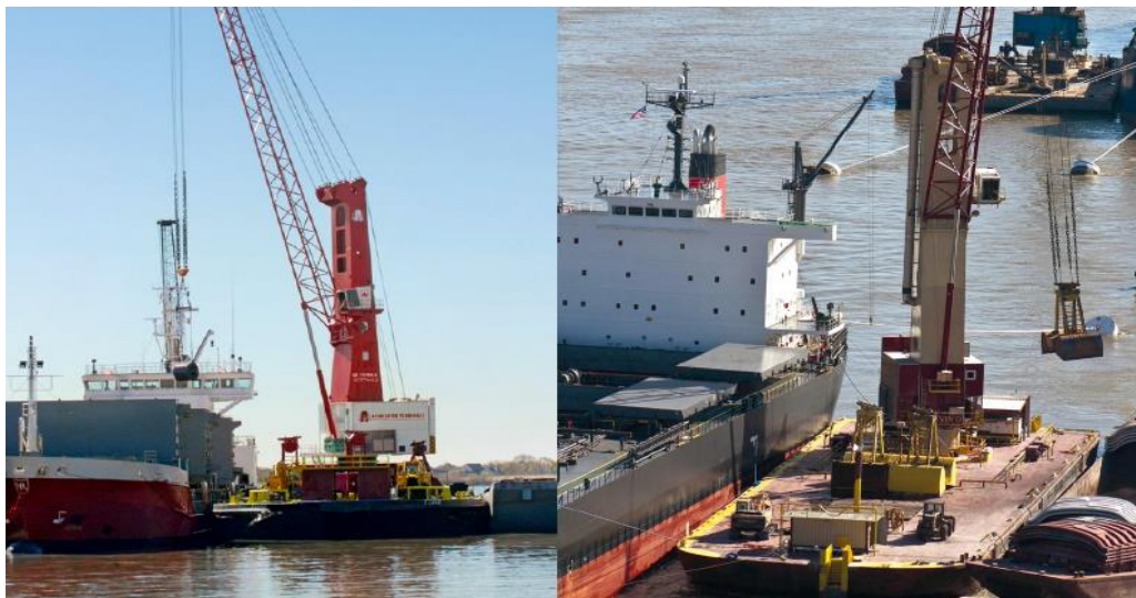
Figure 8: Floating cranes handle cargo in ports with few quay facilities
