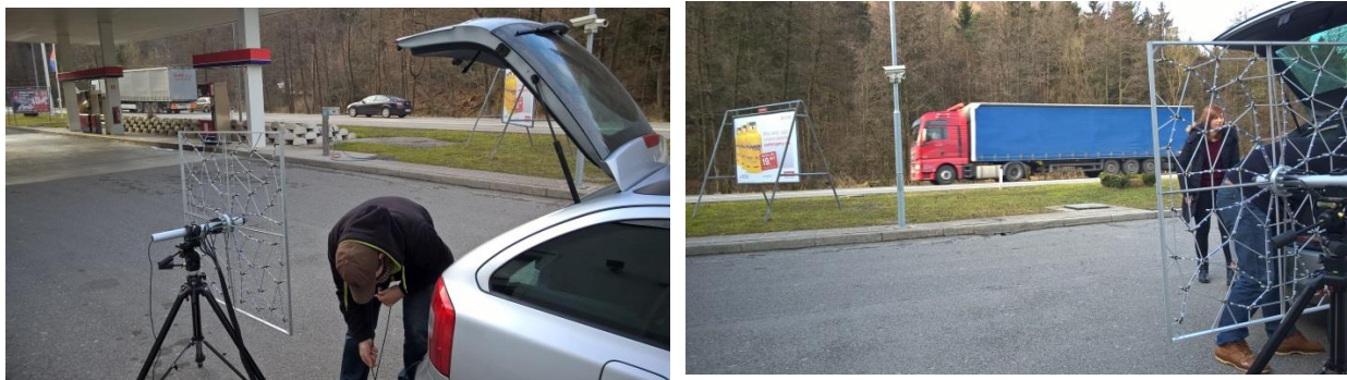
Figure 3: Experimental setup for measurement using an array of 60 microphones (beamforming technique) on the road Velenje – Arja vas
