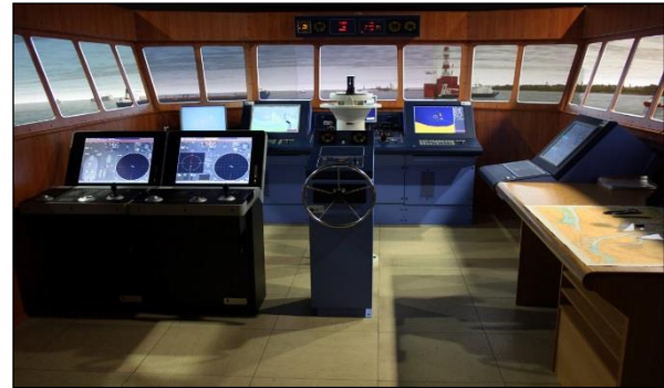
Figure 5: Full Mission bridge of the navigational/ship-handling simulator at MTEC (Marine Traffic Engineering Centre)
