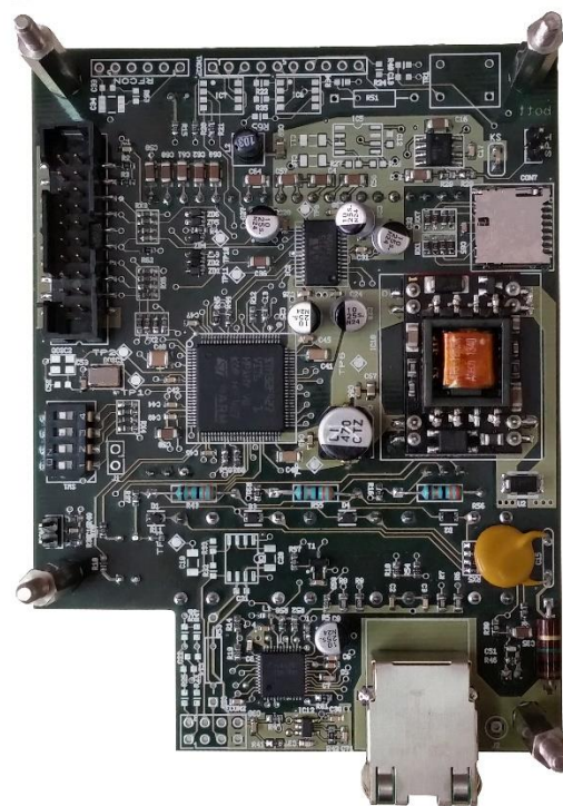
Figure 3: Finished PCB artwork of ship's communication device
