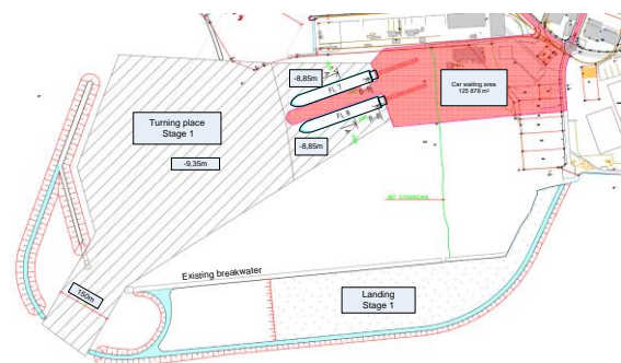
Figure 2: Proposed changes in berths and breakwater arrangements in Port of Ystad (stage 1 only)
