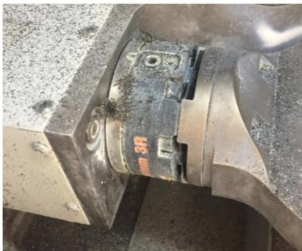
Figure 9 - 10: Steel part (or fragment ) that got magnetized during the cutting processes, and got on magnetic sensors on machine
