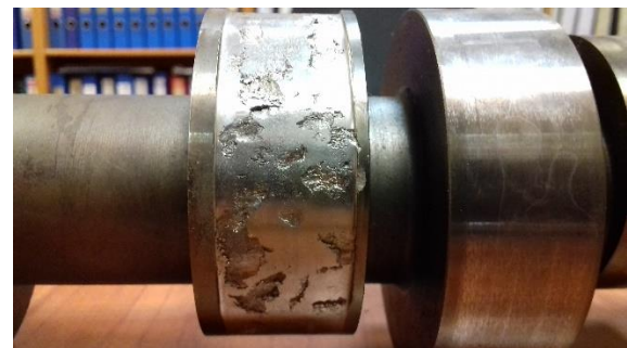
Figure 3: High pressure fuel pump cam destruction
