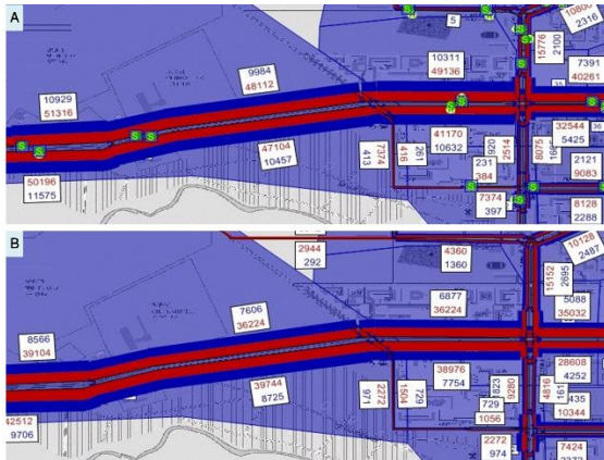
Figure 3: Distribution of transport load according to: a) existing passenger flow and route network; b) predicted passenger flow and upgraded route network
