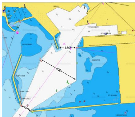
Figure 1: Current dimensions of waterways, infrastructure, and navigational marking inside the Ystad outer port
