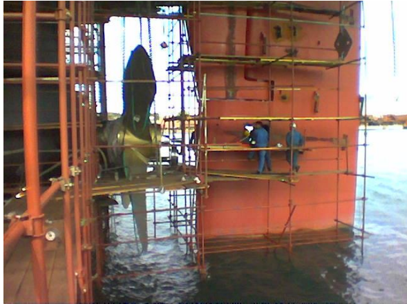
Figure 1: Typical solid 4-bladed fixed pitch propeller immediately after its fitting on its shaft [15]
