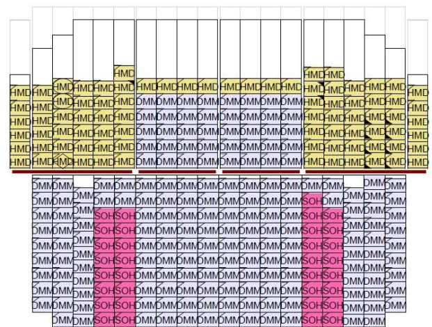
Figure 6: Stowage plan made in SIN for SOH, DMM and HMD
