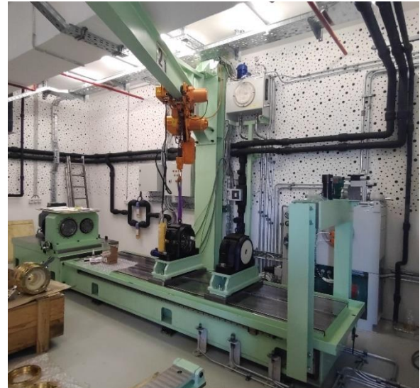
Figure 3: Layout of instrumented test rig prior to the installation of the shaft, test bearing and load module.
