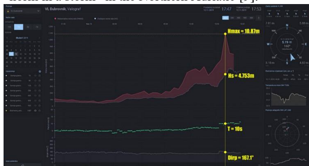
Figure 2: On 12 November 2019 at 16 h, Hydrographic Institute of the Republic of Croatia measured a record-setting wave in the Adriatic. This wave was recorded in the sea area of Dubrovnik near Sv. Andrija islet. Maximum wave height was H_{\max} = 10.87 m, with significant wave height H_S = 4.75 m (sea state 6) and period T = 10 s. The wave arrived from direction Dirp = 167.1^\circ [URL 1].
