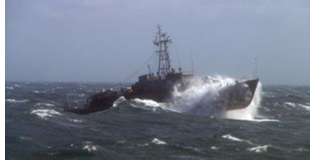
Figure 13: A photo showing the slamming effect
