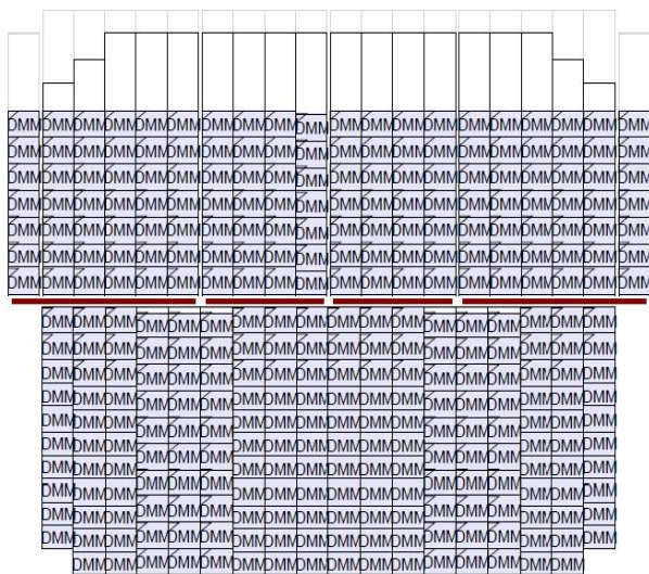
Figure 8: Stowage plan made for a single group of containers – ideal stowage planning
