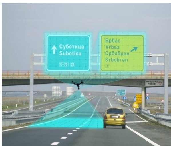
Figure 5: An example of simultaneous collection of data about the characteristics of traffic signs and markings
