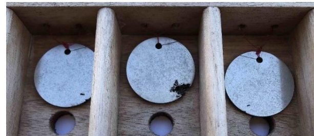
Figure 1: Disc-like NiTi alloy as cast
