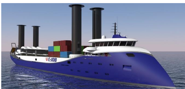
Picture 3: Flettner Freighter by C-Job Naval Architects
