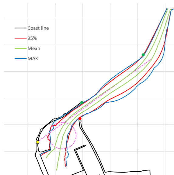
Figure 3: Maneuvering areas of general cargo ship of L=133m on approach to modernized Ustka Port by “Soft-Bank” with limited (preliminary) navigational marking
